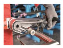
The battery tube polisher ATC 7 achieves the best fine grinding results without great pressure.
