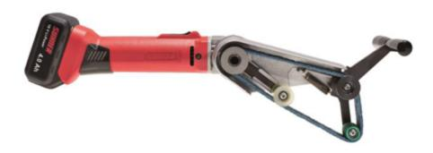
The tube polisher ATC 7 is ideal for tubes up to 45 mm in diameter. Its large wraparound angle of at least 180° ensures fast, efficient work. This battery tube polisher can therefore demonstrate its perfected maneuverability in tight elbows as well. No contact pressure is used for the wraparound. Material can then be removed to a very fine degree, leading to outstanding results.
