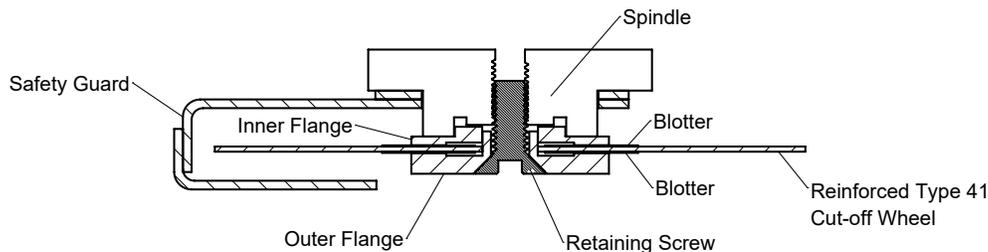
**Note:** Ensure driving tabs of 55364 spindle lock nut are adjacent to and engage slot of 55357 inner flange.
